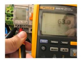
Measure on meter or charger with power off on meter and charger between D+ and D-In general it's easier to measure on the meter. Should be **around 60 Ohm**, correct in this picture.
