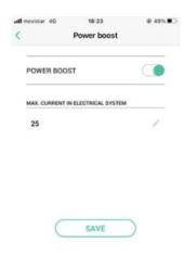
If all correct, connect to charger with bluetooth and Power Boost tile must be selectable, if greyed out there is still no communication with the meter.
